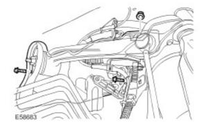
6. Release the shock absorber and air spring assembly.
