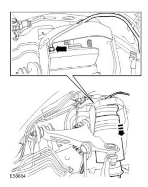
8. Remove the shock absorber and air spring assembly.
