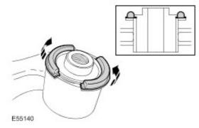
8. Using the special tools, remove and discard the lower arm rear bushings.
