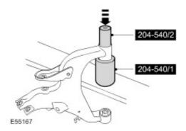
9. Using the special tools, remove and discard the lower arm front bushings.
