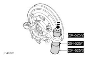
3 . Install the wheel knuckle. For additional information, refer to Wheel Knuckle (64.35.10)
