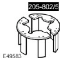
Rear wheel bearing remover/installer 205-802/5
