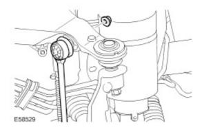
CAUTION: To prevent the wheel knuckle falling outwards and disconnection of the halfshaft inner joint, support the wheel knuckle.
