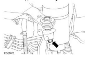
10. Using the special tool, release the upper arm ball joint.
