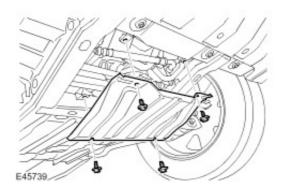
4 . Remove the fender splash shield lower trim.
