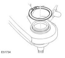
5. Using the special tools, remove the ball joint.
