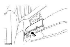
2 . Remove the screw securing the door latch remote release.
